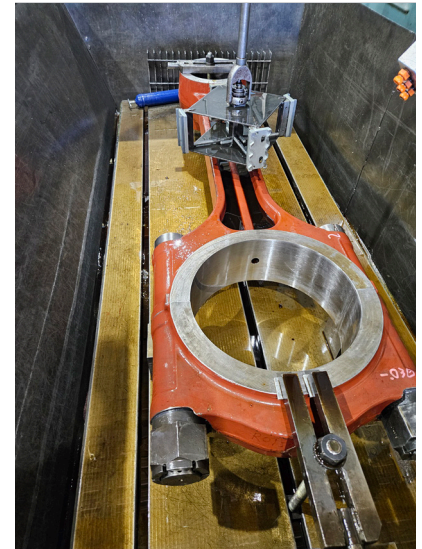
Refurbishing compressor connecting rod to specifications
